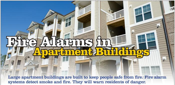
The fire alarm system has many parts that work together. Some of the parts are out of sight. In a fire, smoke detectors sense smoke and activate the fire alarm. Manual fire alarm boxes allow people to sound the alarm. When the fire alarm system activates it will warn residents of danger.
