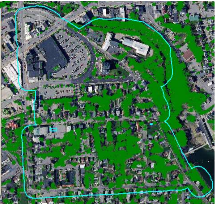
Screen shot of 2018 LiDaR data Analysis in ArcView. Inset graphic displaying summarized pixels over space included to illustrate the software analytical techniques used to quantify 2018 percent tree canopy.
