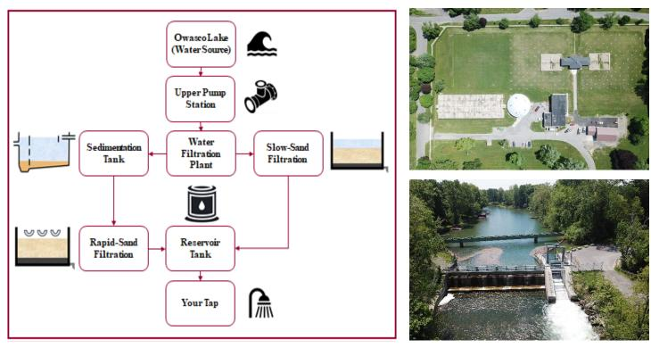
Figure 2. Water Filtration Flow, From Lake to Tap
